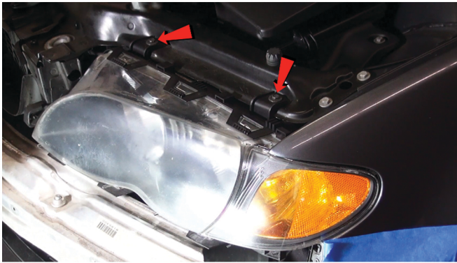
13) Remove [2x] 8mm bolts securing the headlight from above.
