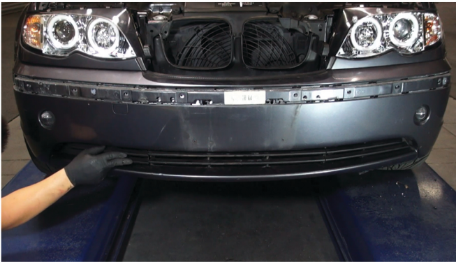
31) Reinstall the lower outer grilles by pressing them back into place.
