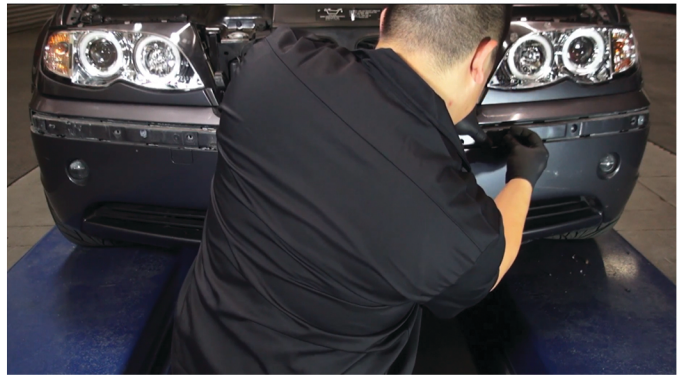
32) Reinstall [6x] plastic retainers to secure the fascia.
