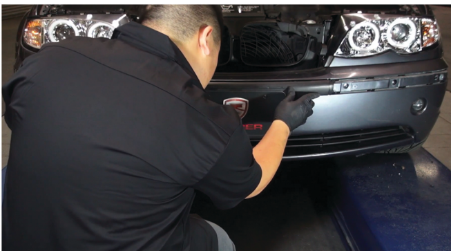
33) Reinstall the center trim piece by seating its retainer tabs.
