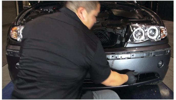
30) Seat the front bumper fascia into the ductwork.
