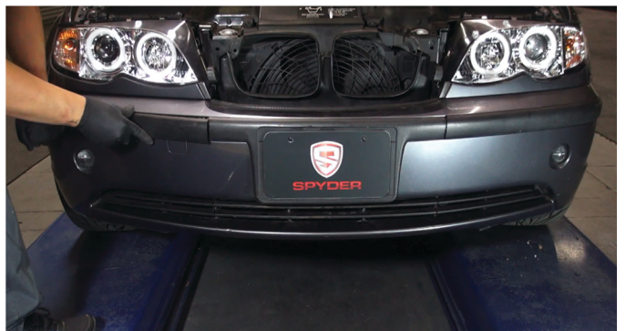
34) Reinstall the outer bumper trim pieces, taking care to seat their retainer tabs. Then slide the trim pieces inward to close the gap between the outer trim and center trim pieces.
