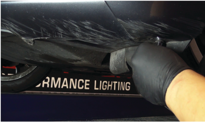
35) Reinstall [2x] 8mm bolts to secure the lower corner of the fascia on each side.
