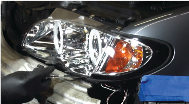
27) Reinstall [2x] 8mm bolts to secure the headlight from below.
