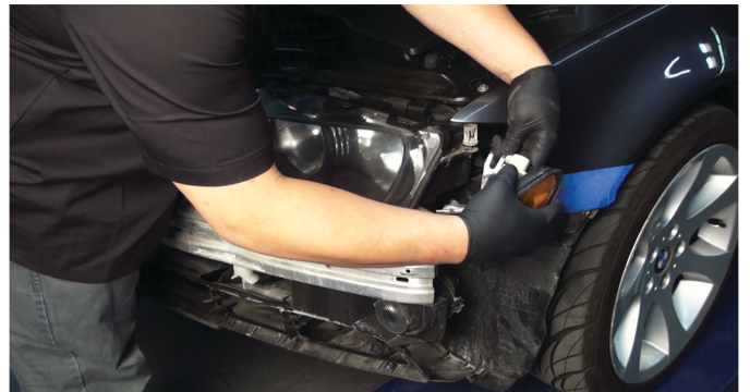
16) Disconnect the corner lamp harness, then remove the corner lamp and set it aside.
