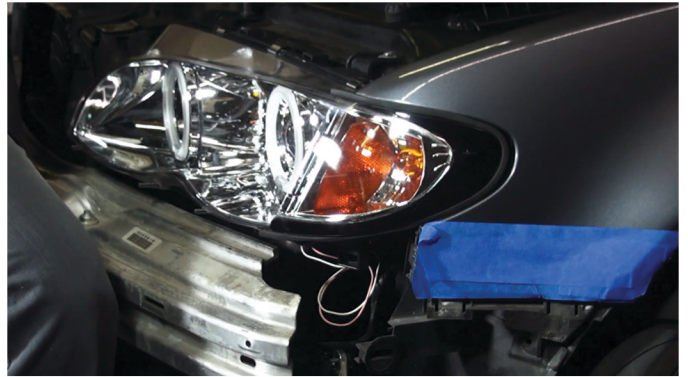
26) Reinstall [2x] 8mm bolts to secure the headlight from above.
